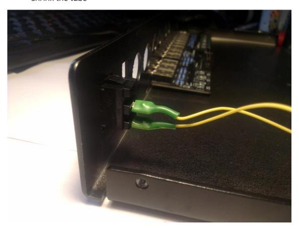
• solder the other ends of the cable to the 2 contacts of 'S33' on the PCB. It does not matter which cable goes to which side.
