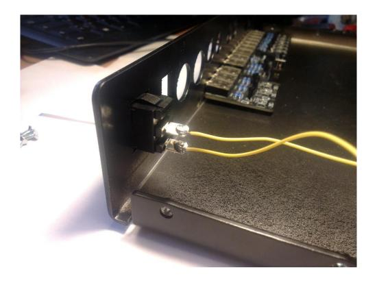
• Put the shrinking tube on the a power switch contacts
