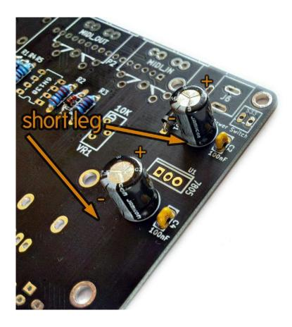
solder the 100uF cap below the mainboard connector P1. Once again, this is a polarized part. Short leg to round pad.
