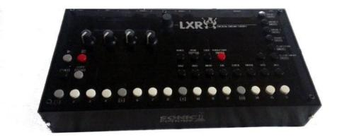
As a last step, you may now tighten all the screws of the enclosure. Not too firm, or you may crack the plastic, but the screws should not move when you shake the enclosure. Don't forget to attach the 4 rubber feet in the 4 corners of the bottom panel.
