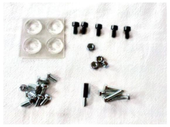
The content of the bag is 4 x sticky rubber feet 5 x black hex screw 4 x M3 nut 1 x 10mm standoff 4 x long M3 screw 13 x short M3 screw
